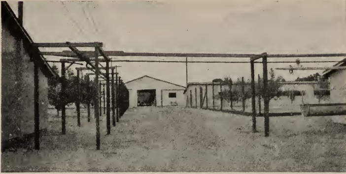
Fig. 64.—A manufactured, all metal litter carrier in use on a large poultry farm in San Luis Obispo county.
